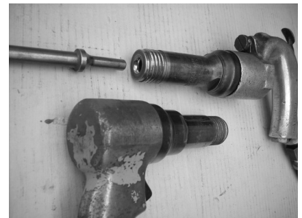
Above: Bottle opener made with air hammer Below: Socket must match the tool bit!
